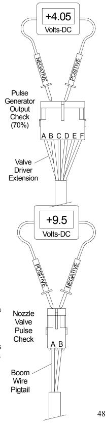
Make the same measurement on an adjacent nozzle valve. The wire color in position B should change from white to green or green to white.
