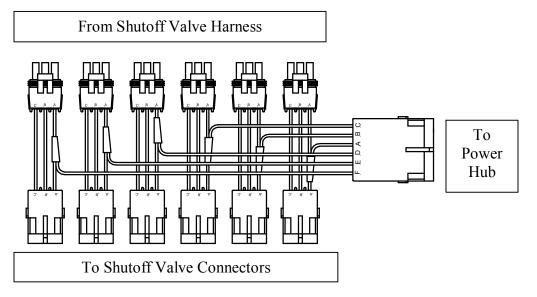
If no shutoff adapter is available to match the sprayer, the boom shutoff pigtail (PN: 118602-001) can be used to hand wire the shutoff signals. Connect the boom-1 shutoff signal to pin-A, boom-2 to pin-B, etc. Consult the SharpShooter wiring schematic for additional information.
