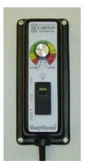
Turn the Rotary Switch knob to 40 and turn on SharpShooter in PSI Mode by flipping the switch upward toward the Rotary Switch knob. Observe SharpShooter adjust the pulse duty cycle to achieve 40psi. The spray rate controller may need to be adjusted to put SharpShooter in a practical control range.
