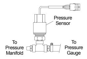
Whenever possible, Capstan recommends that the Pressure Sensor be installed vertically and with the sensor pointed upwards. This helps to keep debris from settling in the sensor.
