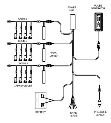
Shorten the power wire to the appropriate length and terminate the wire with the battery ring terminals provided. If a battery fuse kit is provided, crimp it onto the red power lead in lieu of the ring terminal. It is recommended to use battery terminal corrosion inhibitor to prevent salt buildup and extend the life of the battery terminals.
