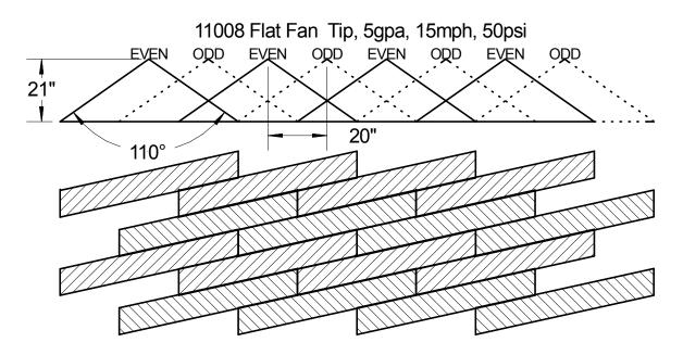
In this example, each nozzle is spraying 1/3 of the time, but adjacent nozzles alternate and overlap to fill in the areas between nozzles. As the sprayer increases speed, rate or boom
