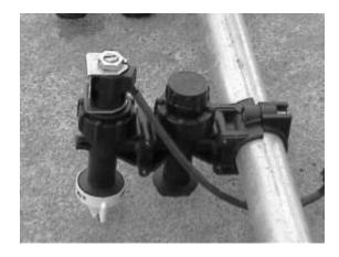
Plug the nozzle valve into the boom wire and secure the wire with a nylon cable tie.
