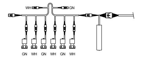
Since two boom sections are generally started at the center of the boom and boom wires extended to the left and to the right, there will be two "even" pulse valves adjacent to each other. A nozzle alternator can be placed between the Valve Driver and boom wire to "flip" the odd/even pulse alternation (the colors, of course, will not flip, so it is important to remember that the nozzle alternation has been flipped).
