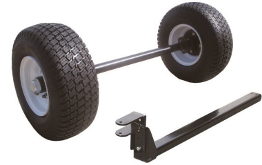
40 & 60 Gallon Trailer Kits Axle & tongue assembly 40 gallon kits have bushing bearings and 15x6-6 tires 60 gallon kits have four bolt hubs, roller bearings, and 16x6.5-8 tires Must be used with 40 & 60 gallon tank skid 40 Gallon Kit SSFK-4000SL-MM 60 Gallon Kit SSFK-6000SL-MM
