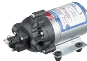
12 VDC Internal Bypass 1.8 GPM Demand Pump 45 PSI, Electrical Package 8007-543-850
